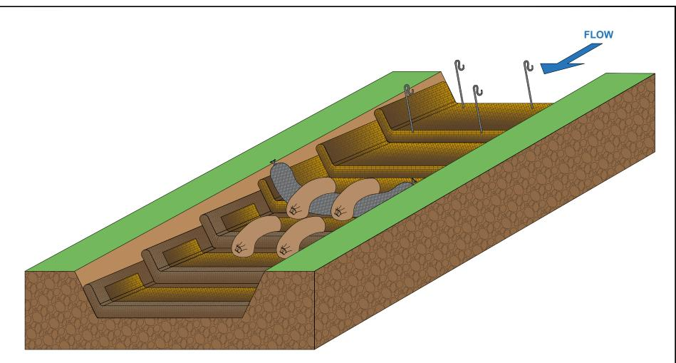
Silt Wattle - a permeable barrier that moulds to the shape of the ditch, slows the flow and improves treatment
