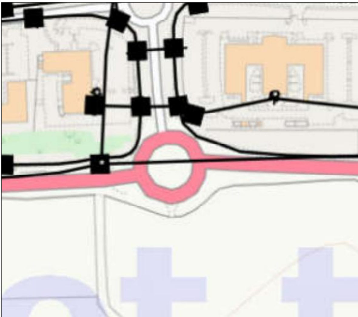
Figure 5.5.4 – Existing underground Openreach chambers and ducts in the vicinity of the existing roundabout
