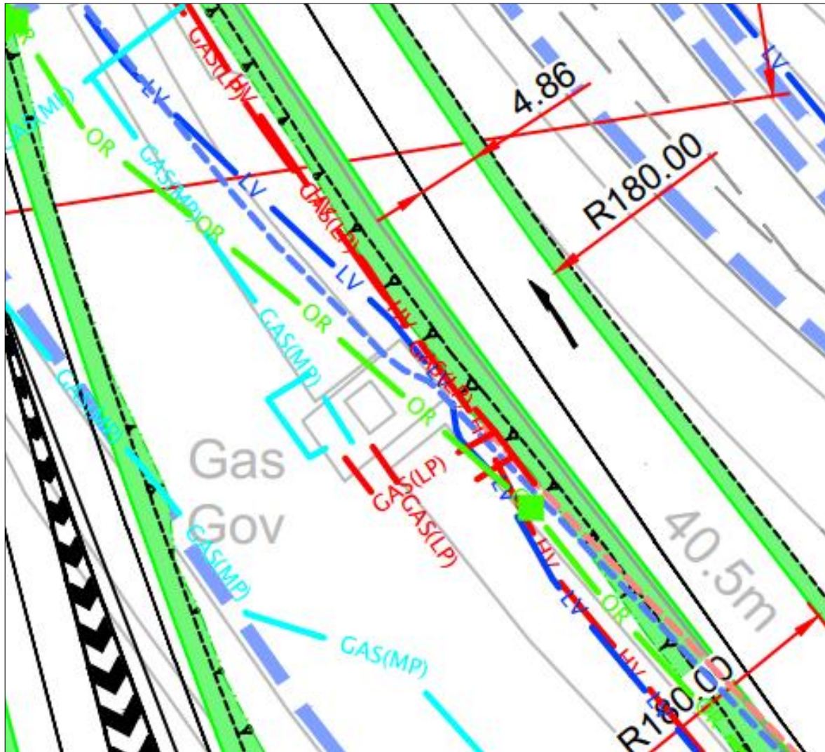
Figure 5.13.7 – Existing gas governor adjacent to the A50
