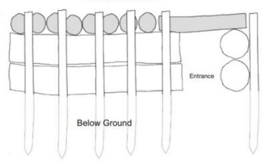
Place smaller logs and branches along the top of the chambers to form a roof. Fill any gaps with smaller pieces of wood for weather protection and prevent light gaps.
